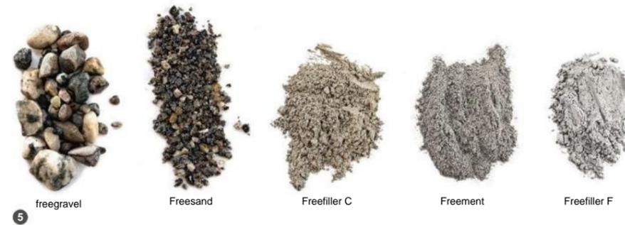
tor, at the Dutch company Smart Circular Products/Urban Mine (*Betoniek Vakblad* 2020/1 'An overview of innovative recycling methods' [9]). With this separation technique, from which five product flows arise, the adhered cement stone can be removed from the original sand and gravel by shear forces. The powdered cement stone is released as a separate production flow and can, for example, be used directly in concrete as a filler.
