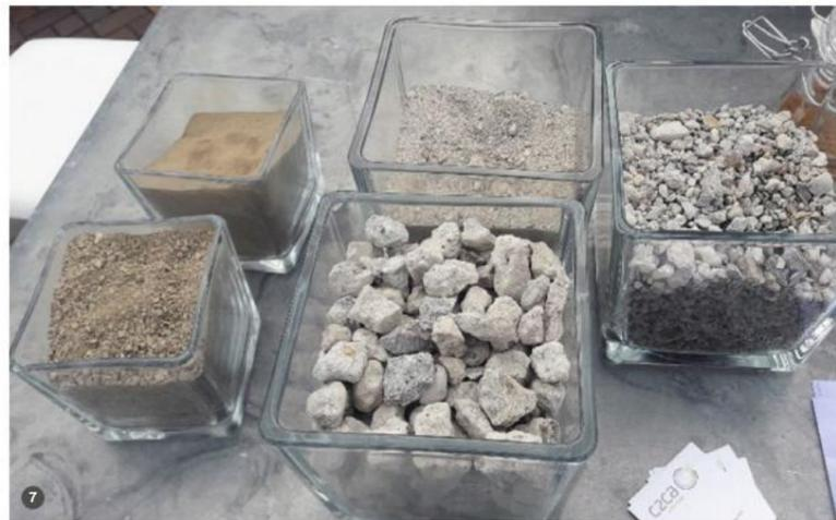
The sand and gravel have an 80% clean surface. It is estimated that this will allow higher replacement percentages than on the basis of traditional materials, but lower than the two methods mentioned above. The cement stone powder can also be used here as a filler.
